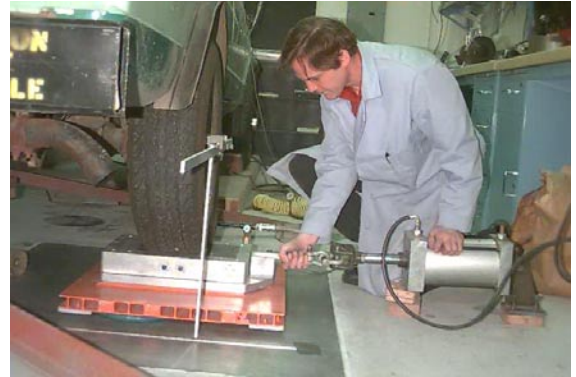
Figure 6: CRREL Test Apparatus for Measuring Tire Lateral Stiffness
