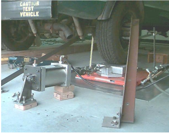
Figure 3: CRREL Test Apparatus for Measuring Tire Foundation Stiffness
